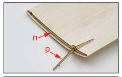
Pay attention to adjust the wing while pasting the wing ribs in order to avoid the wing distortion.
