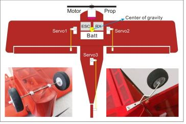
4.01 Assemble electronics as what show in the picture, then adjust central weight of the plane
