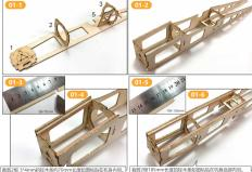
裁剪2根 3\*4mm的轻木条约70mm长度如图粘贴在机身内侧 Cut 2 pieces of 3\*4mm balsa strips with 70mm length and paste inside the fuselage as shown.
